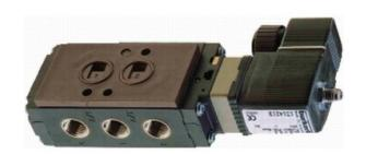
The Type 6519 Namur is a valve for plant technology that switches reliably even with full restriction. The valve can be operated as a 5/2 or 3/2—way valve through the various mounting positions of the changeover plate on the side.
