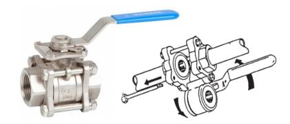
They are of floating ball construction whereby the ball is free to move horizontally inside the body, the movement induced by line pressure acting on the ball. The downstream seat, opposite the pressurised side of a closed valve, carries the load exerted by the line pressure on the ball, whilst the upstream seat is subject to little load or wear. For this reason it is sometimes possible to increase the seat life by swapping these seats around.
