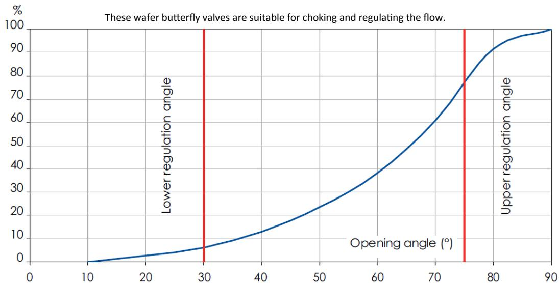
**Flow Chart (Kv in m<sup>3</sup>/hr at 1 bar pressure drop)**
