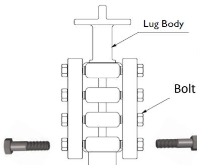
Lugged & tapped butterfly valves are suitable for end of line service.
