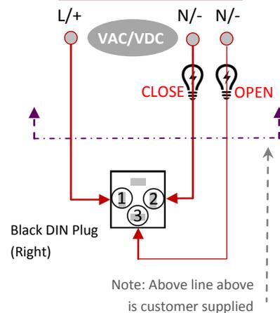
In J+J electric actuators all electrical connections are made externally using the external DIN plugs supplied with the actuator. There is no need to remove the valve actuator's cover to connect electrically. There are no terminals internally to connect to.
