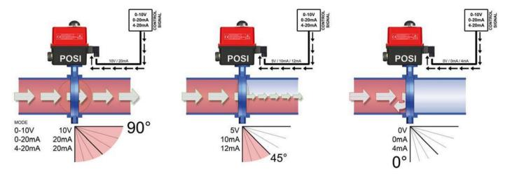
Note: Allow a safety factor of torque x 2 when sizing Valpes modulating actuators
