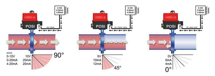
Note: Allow a safety factor of torque x 2 when sizing Valpes modulating actuators
