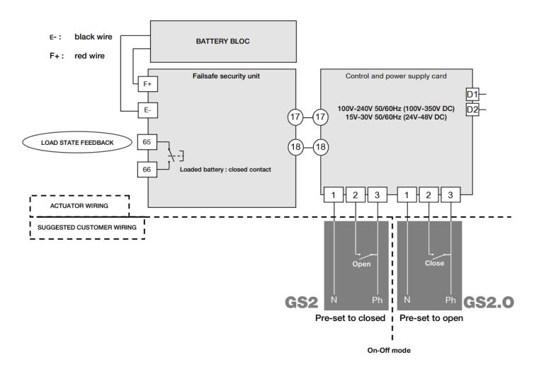
Note: Pre set position is factory set and can not be changed within the actuator, fail open and fail closed versions are different actuators.
