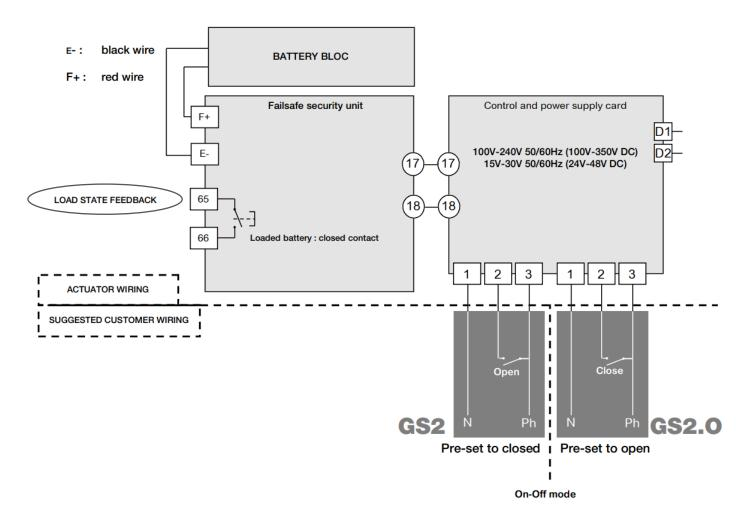
Note: Pre set position is factory set and can not be changed within the actuator, fail open and fail closed versions are different actuators.
