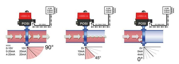
Note: Allow a safety factor of torque x 2 when sizing Valpes modulating actuators
