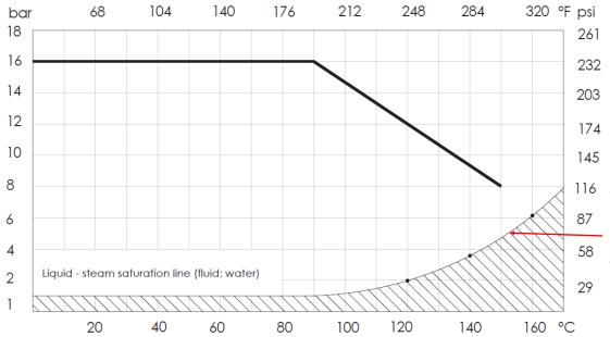
145 Liquid-steam separation line. Do not use these valves if the application is in the hatched area below the line.
