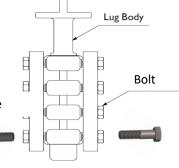
Fully lugged and tapped body, suitable for end of line service
